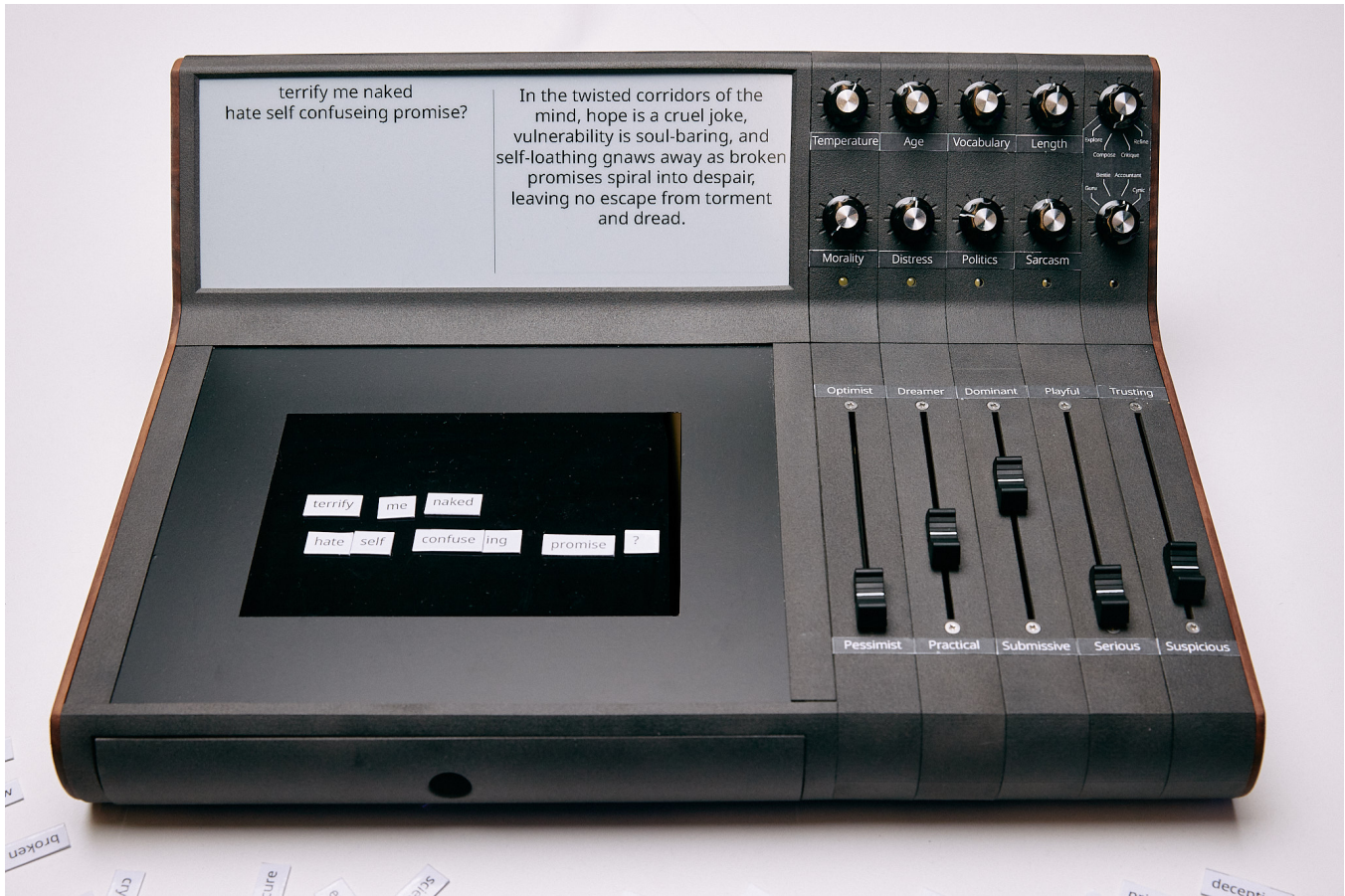
Figure 2: The Memetic Mixer, used as a design probe with four creative practitioners. To interact with the device, word tiles are placed on the dark rectangular region and the e-screen at the top displays words as they are placed (left) and the device’s response to them (right). The bottom right faders represent personality traits, while the knobs above provide different ways to direct the LLM.
